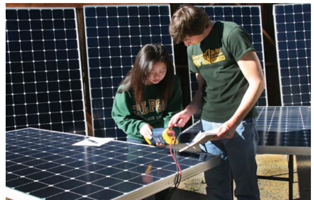
Students testing donated photovoltaic panels prior to installation. Photo: CPSLO.
