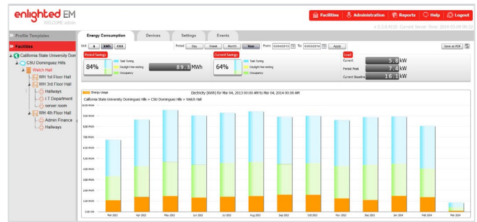
System interface screen from Enlighted displaying real-time, monthly and annual energy savings at Welch Hall. Image: CSUDH.
