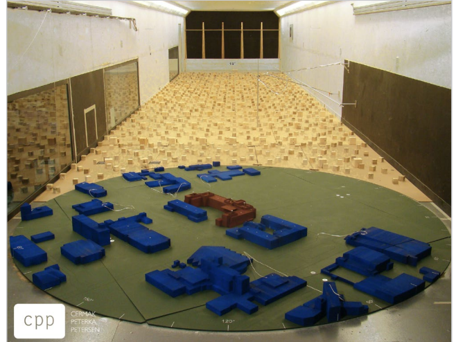
Wind tunnel model used to establish minimum safe stack exhaust velocities. Image courtesy of CPP Wind Engineering.
